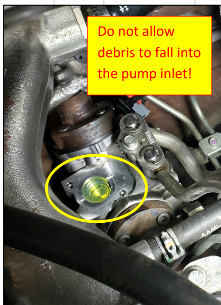
Figure 9: FCA Removed (no debris)
