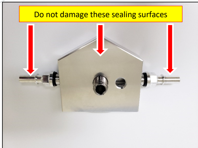
Figure 1: Torque Fittings to 120 in-lb (10 ft-lb)
