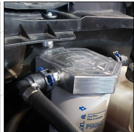
Figure 12: Filter Head Installed – 2017+
