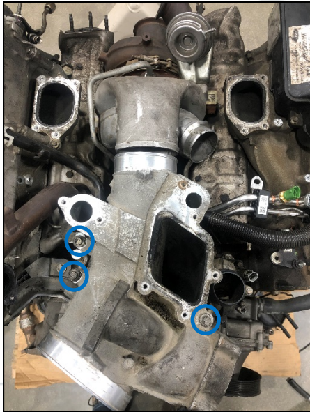
Figure 5: Lower Intake Bolts
