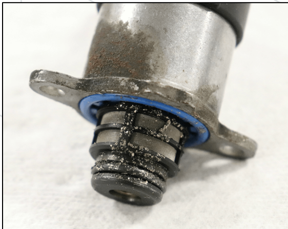
Figure 7: Failing CP4 FCA without Bypass Kit installed
