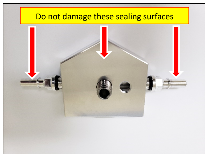
Figure 1: Torque Fittings to 120 in-lb (10 ft-lb)
