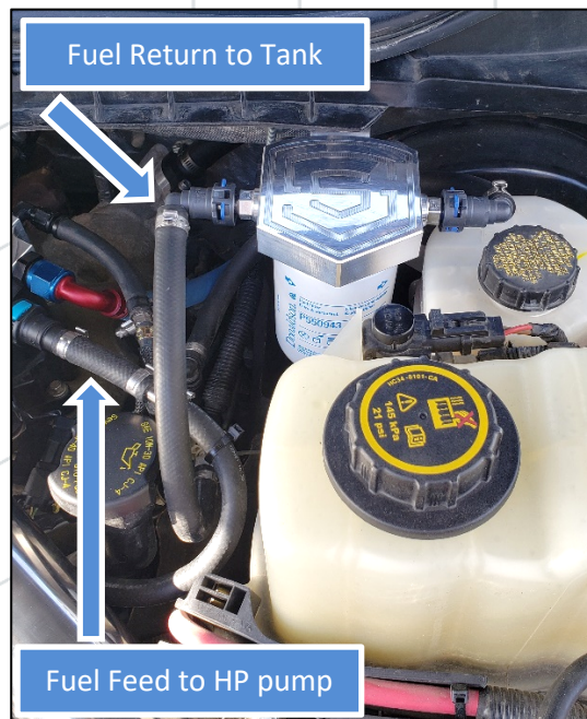
Figure 7: Left Side hose installation (2017+)
