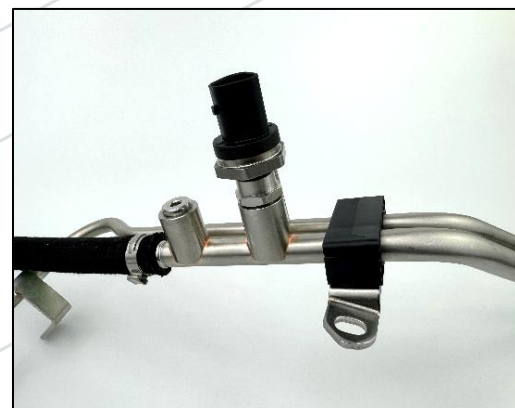
Figure 32: 2015-2019 (Plug, Adapter + OEM Sensor)
