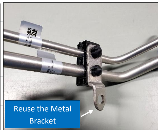
Figure 34: Reuse metal OEM bracket
