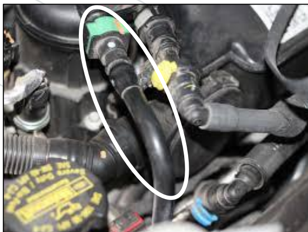
Figure 9: Fuel line is removed and not reused
