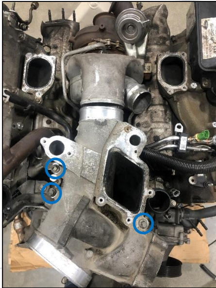
Figure 5: Lower Intake Bolts
