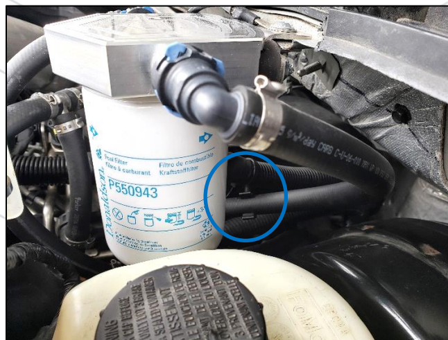
Figure 5: Zip tie clip placement
