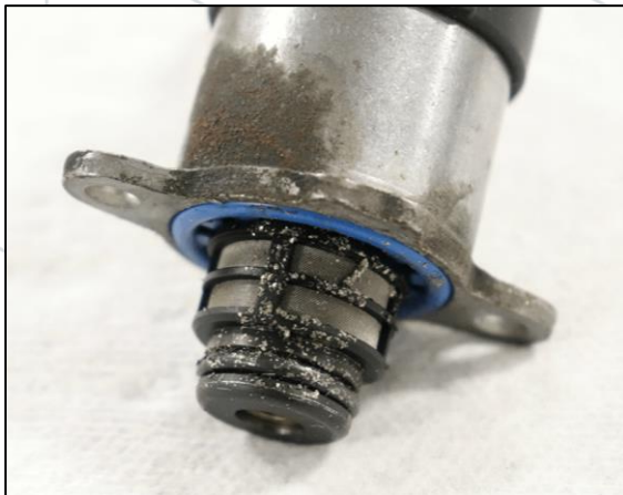
Figure 7: Failing CP4 FCA without Bypass Kit installed
