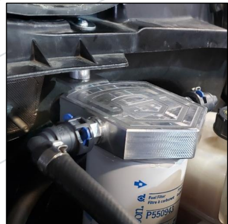
Figure 12: Filter Head Installed – 2017+
