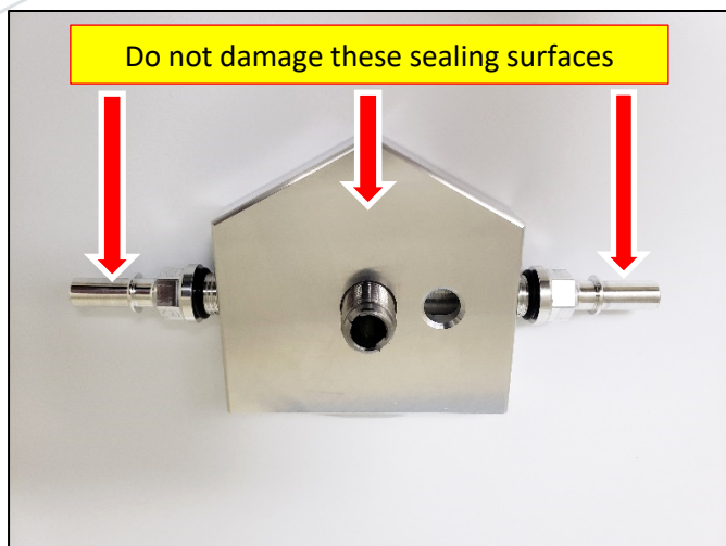
Figure 1: Torque Fittings to 120 in-lb (10 ft-lb)
