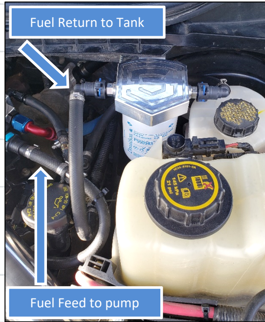
Figure 7: Left Side hose installation (2017+)
