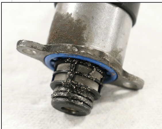
Figure 7: Failing CP4 FCA without Bypass Kit installed
