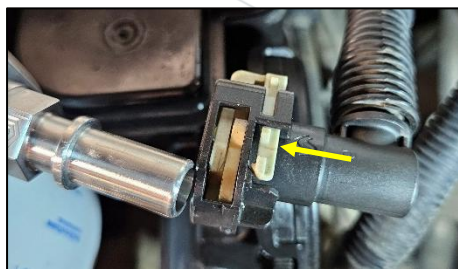
Figure 14: Lock Tab Middle Position
