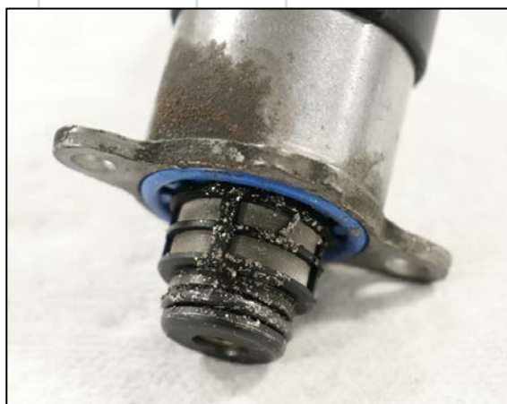
Figure 7: Failing CP4 FCA without DPK installed
