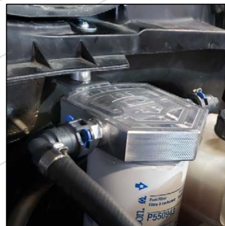
Figure 12: Filter Head Installed – 2017+
