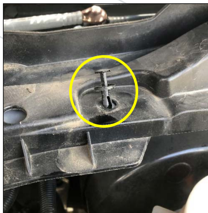
Figure 10: Remove plastic fastener
