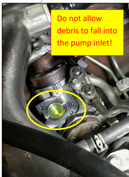
Figure 9: FCA Removed (no debris)
