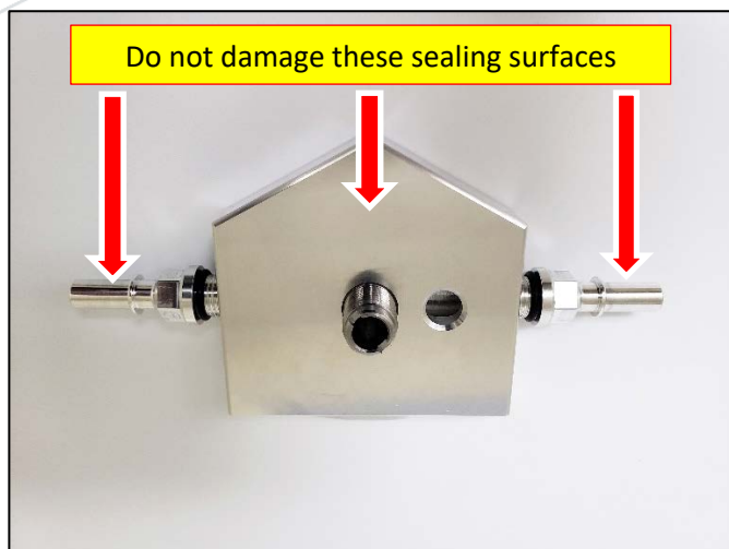
Figure 1: Torque Fittings to 120 in-lb (10 ft-lb)
