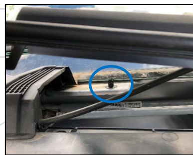
Figure 9: Clip under the cowl x2
