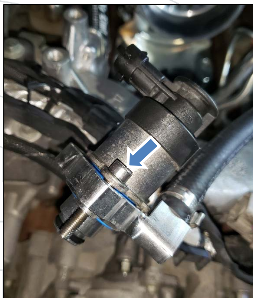
Figure 11: Subassembly Block, FCA, and front bolt
