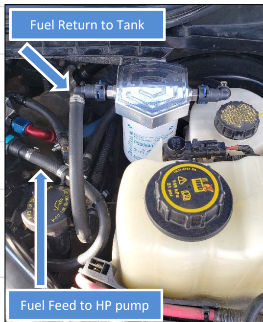
Figure 7: Left Side hose installation (2017+)
