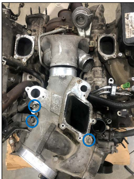
Figure 5: Lower Intake Bolts
