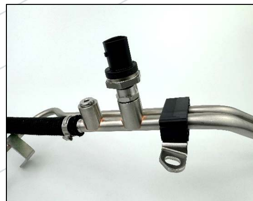
Figure 32: 2015-2019 (Plug, Adapter + OEM Sensor)
