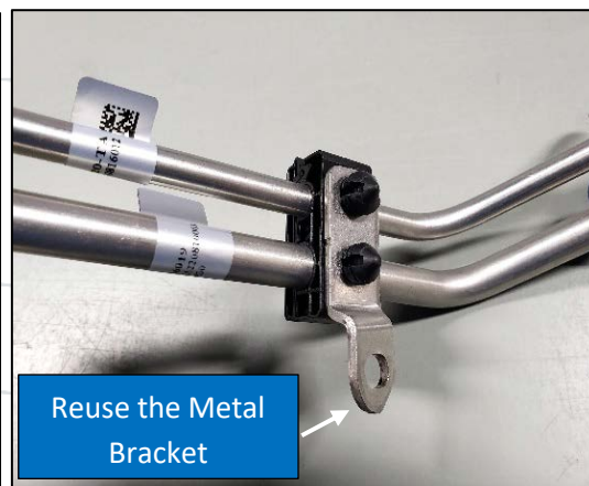
Figure 34: Reuse metal OEM bracket
