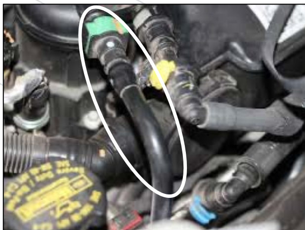
Figure 9: Fuel line is removed and not reused
