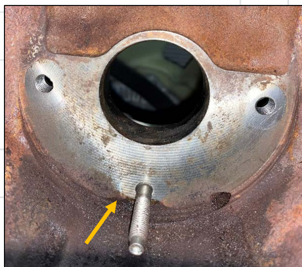
Figure 22: Pump Mounting Surface Cleanliness
