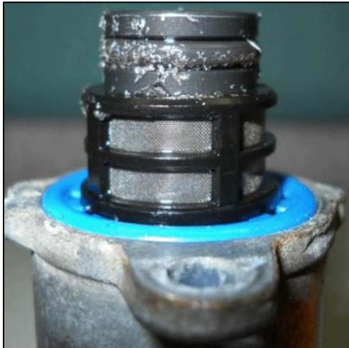
Image 2 – Example of condition from pump failure
