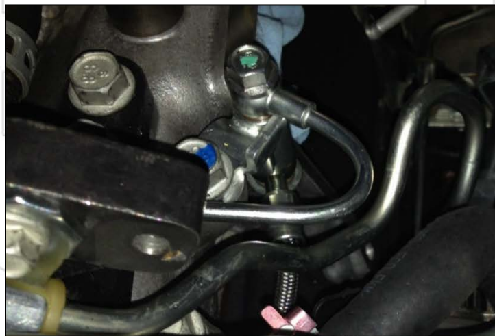
Image 10 – hydrocarbon injector line installed
